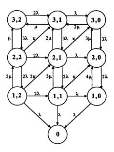
Figure 1: State Transition Diagram for Available Copy with 3 sites and 2 spares
