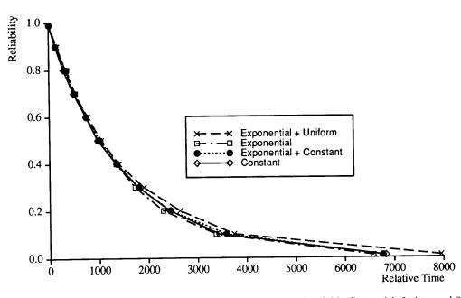
Figure 2: Compared Regeneration Distributions for Available Copy with 3 sites and 2 spares
