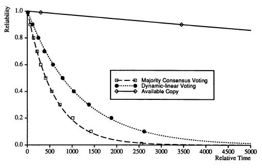
Figure 4: Compared Reliability of AC, DLV and MCV:  $\kappa = 10.0, \lambda = 0.1, \mu = 1.0$
