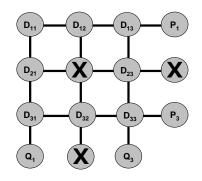
Fig. 3. One of the nine possible triple failures that will result in a data loss.
