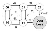
Fig. 11. State transition probability diagram for a stripe consisting of three data disks and two check disks.
