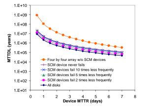
Fig. 12. Impact of SCM reliability on the Mean Time To Data Loss of a set of four RAID level 6 arrays.
