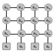
Fig. 6. A partially declustered two-dimensional RAID array with twelve disks and four SCM devices.
