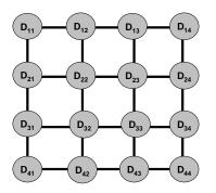
Fig. 4. A fully declustered two-dimensional RAID array with sixteen disks.
