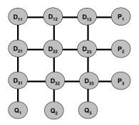
Fig. 2. A two-dimensional RAID array with nine data disks and six parity disks.
