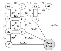
Fig. 8. Simplified state diagram for a partially declustered two-dimensional RAID array with twelve disks and four SCM devices.
