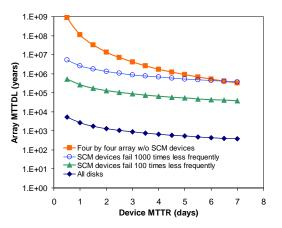
Fig. 13. Impact of SCM reliability on the Mean Time To Data Loss of a set of nine mirrored pairs each consisting of a disk and an SCM device.
