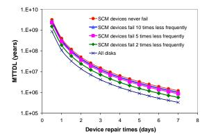
Fig. 9. Impact of SCM reliability on the Mean Time To Data Loss of the array.
