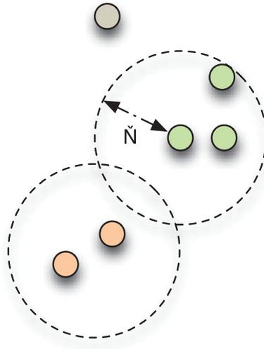
Fig. 2. Each incoming access is compared to the preceding access to determine whether it falls within the neighborhood ( $\check{N}$ ) to be in the same group. If it does not, a new group is formed with the incoming access.
