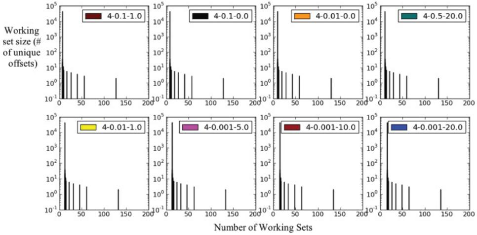
Fig. 12. The bag-of-edges technique run on **msr** data with varying offset and time scaling. Each graph is labeled as number of levels: offset scaling factor, time scaling factor. The resulting group distribution for a given level is very similar regardless of the input parameters.
