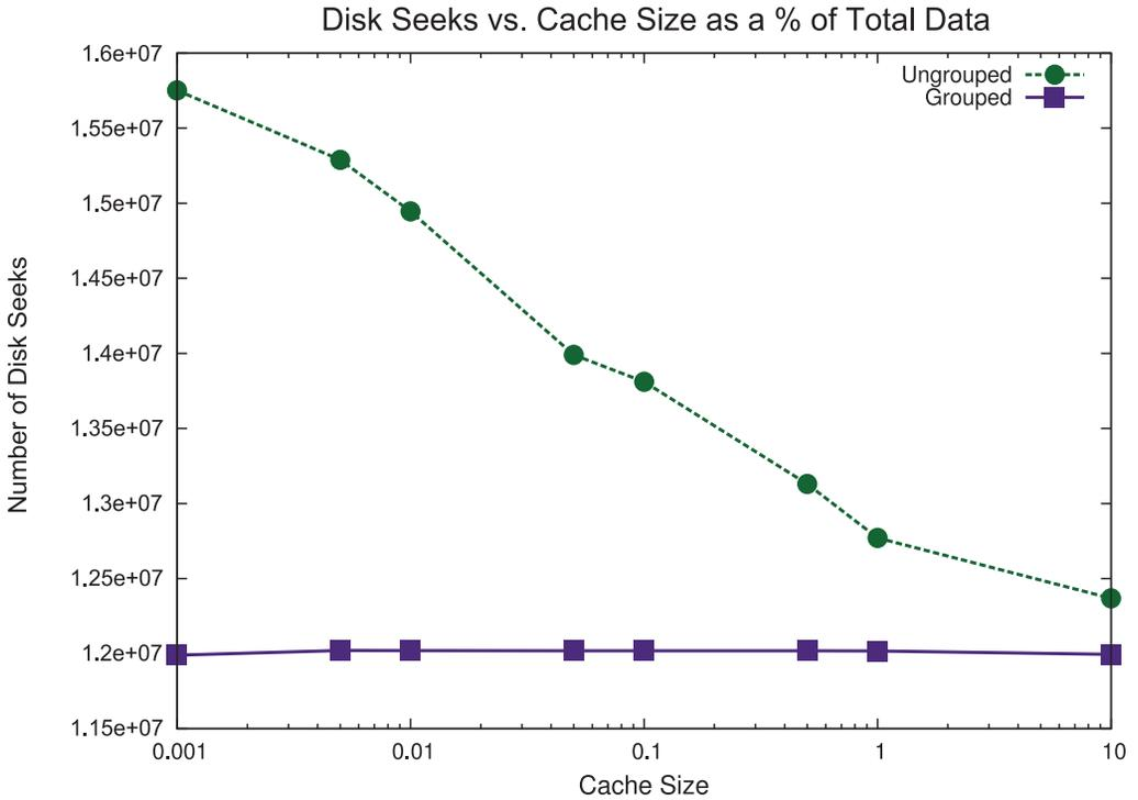
Fig. 13. Disk seeks in grouped versus ungrouped data for the **fu** trace with an LRU cache. Note that with small cache sizes, grouping has an outsized advantage that decreases as more data is simply left in the cache.
